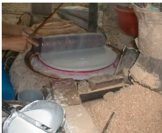
Figure 3: Separating rice paper from a cotton fabric
