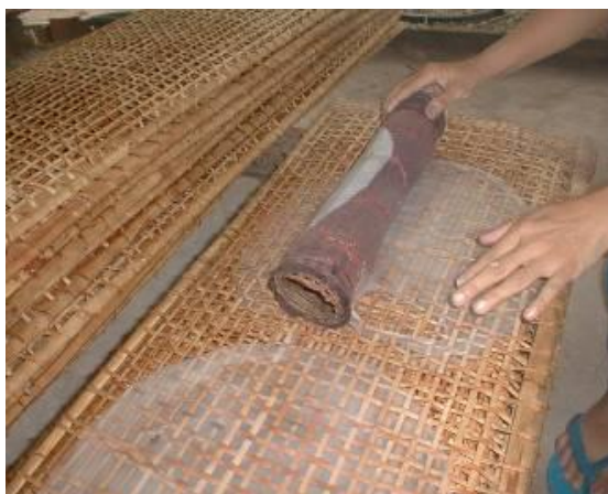
Figure 4: Hanging rice paper on a bamboo woven mat
